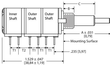
As shown, Outer Shaft operates sections 1 & 2, Inner Shaft section 3
