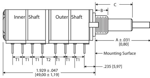
As shown, Outer Shaft operates first two sections
