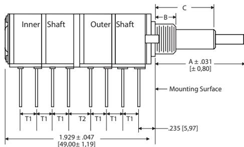
As shown, Outer Shaft operates first two sections
