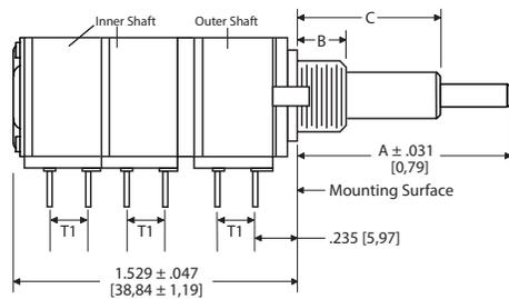
As shown, Outer Shaft operates First Section
