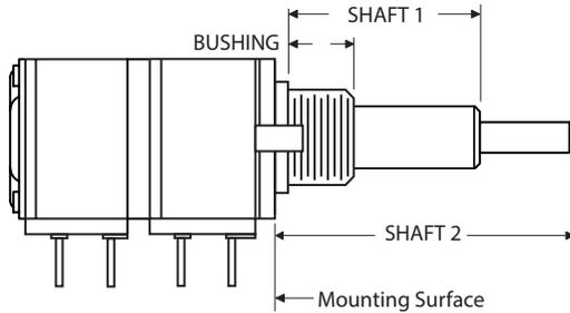
The first section of the potentiometer is referred to as the "Panel Module". All designs begin with a panel module and may be followed by other modular components such as resistor modules, rotary switches, spacers and finally a rear plate.
