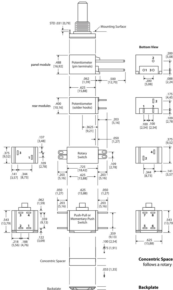
All drawings are shown with 3/8" dia. bushing with 1/4" dia. shaft.
