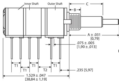
As shown, Outer Shaft operates First Section
