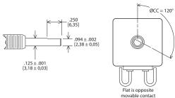
Flat will extend to within .031 [0,79] of mounting bushing where shaft length will not permit standard flat.
