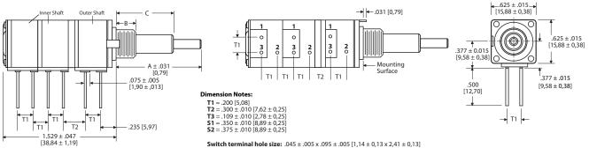
As shown, Outer Shaft operates First Section
