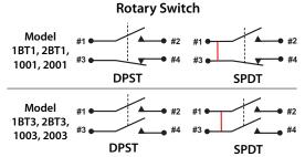
Diagram shows shaft in detent position. Connect terminals #1 and #3 for SPDT Red wire shown here can be added by user. Maximum of 2 rotary switches per shaft.
