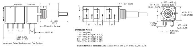
15A-PC - Triple Potentiometer, Concentric Shaft, Solder Pins
