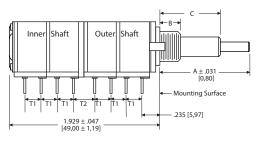
As shown, Outer Shaft operates first two sections
