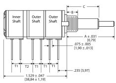
As shown, Outer Shaft operates sections 1 & 2, Inner Shaft section 3
