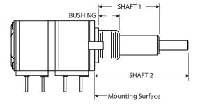
The first section of the potentiometer is referred to as the "Panel Module". All designs begin with a panel module and may be followed by other modular components such as resistor modules, rotary switches, spacers and finally a rear plate.
